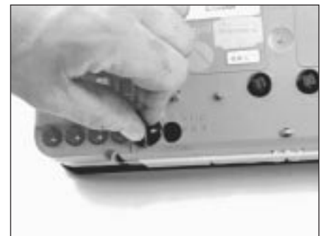
10.5 Turn the plastic knobs to release the back of the cluster (some models use screws)
