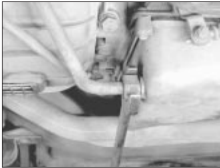
28.5a Unscrew the dipstick tube collar
