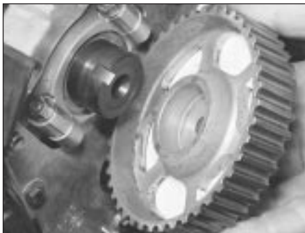
10.10 Removing the camshaft sprocket on the M40 engine
