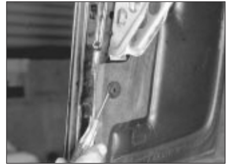
10.8b . . . prise the retainer out
