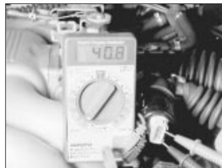
21.21 Check the idle air stabiliser valve resistance on the two outer terminals on later Motronic systems - it should be about 40 ohms
