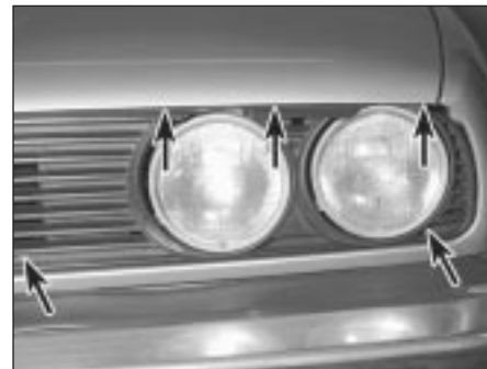
9.2b Side grille screw locations (arrowed)
