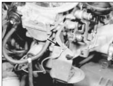
11.5 Remove the screw, and disconnect the carburettor earth cable (arrowed)
