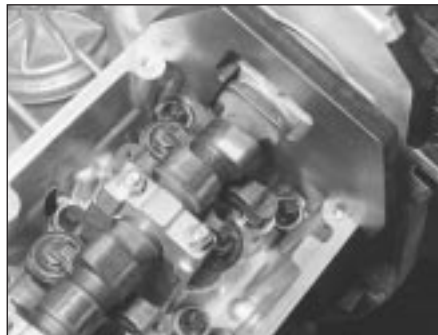
10.11b The BMW camshaft-holding tool in position on the M40 engine
