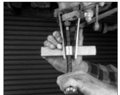
4.7b You can separate the thrust arm balljoint from the steering arm with a puller . . .
