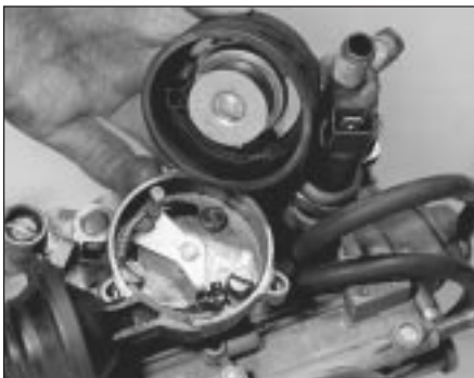
12.18 Remove the automatic choke cover, at the same time disengaging the bi-metal spring from the control lever
