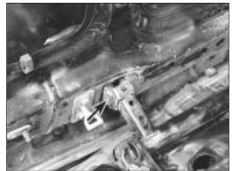
10.12 Unscrew the hinge through-bolts (arrowed)
