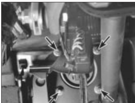
8.10 Remove the four mounting nuts (arrows) and withdraw the servo unit from the engine compartment (left-hand-drive model shown)
