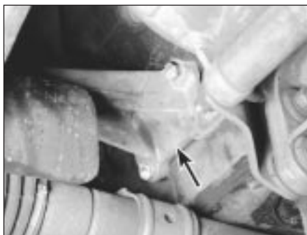
17.5 Lever gently between the block and the engine mounting attachment point (arrowed) - if there is movement, tighten the bolts
