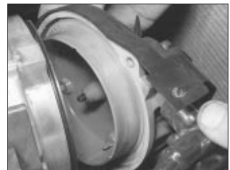
9.6a Unbolt the distributor cap (M40 engine) . . .
