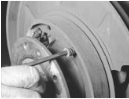
12.7c Remove the shoe hold-down springs
