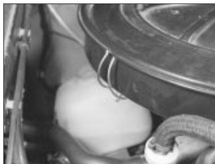
8.2a Release the air cleaner cover spring clips . . .
