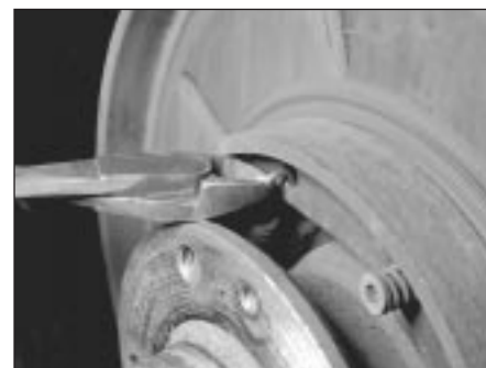
12.7b Remove the upper shoe return spring
