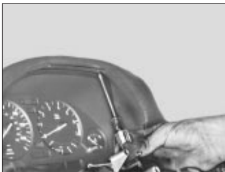
10.3 Use a Phillips screwdriver to remove the instrument cluster retaining screws
