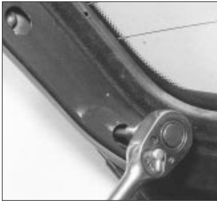
14.14 Unscrewing the hinge mounting bolts (5-Series)
