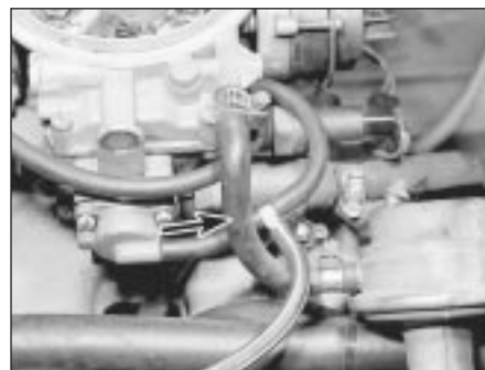
11.8 Disconnect the fuel supply hose (arrowed)
