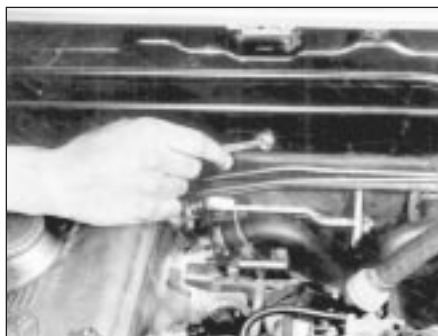
9.2a To get to the heater blower motor, the access panel must be removed - a fastener from the front and . . .
