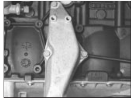
7.3 Engine left-hand mounting bracket - M40 engine
