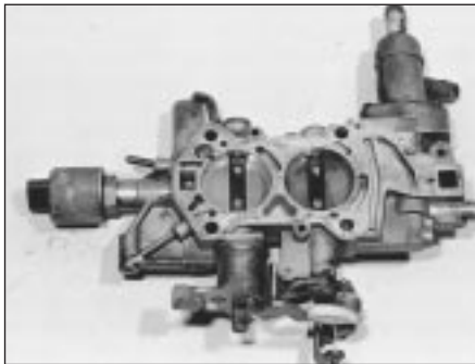
12.11a Throttle housing removed from the carburettor
