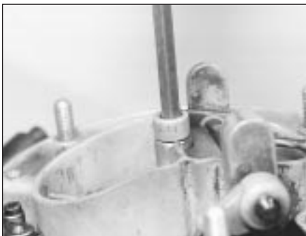
12.4 Using an Allen key to remove the carburettor cover centre bolt
