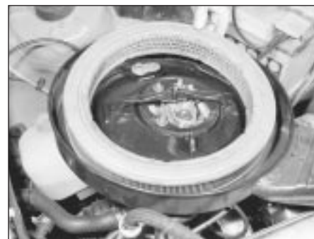
8.3 Remove the air cleaner element, and wipe clean the body and cover
