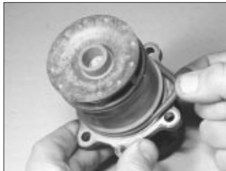
7.23 Fit a new O-ring on the M40 engine water pump
