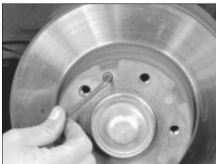
5.6a Remove the disc retaining screw ...
