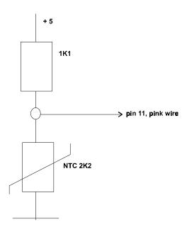
The above circuit is not realistic. The input of the ECU (pin 11) can be connected to an existing temperature input with the following voltages:
